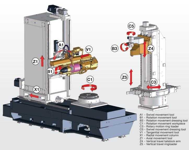
The grinding head is based on a proven design principle with spindle speeds up to 12,000 rpm. Its high thermal stability is a prerequisite for profile grinding. Active tool clamping on both ends guarantee high tool rigidity. Therefore, a cutting speed of 100 m/s is easily achievable.
